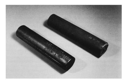
A side by side comparison of both a sand cast bar and a Versa con–cast bar shows why machinist prefer the as cast finish of the VERSA–BAR product. The continuous casting method offers a superior surface finish and virtually eliminates internal porosity and centerline shrinkage.
