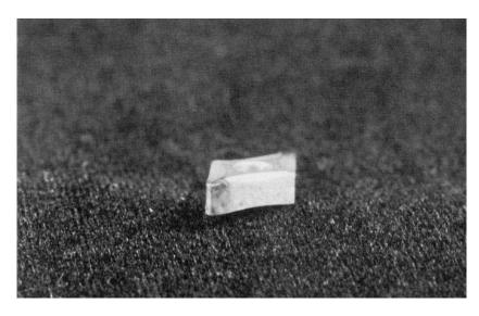
This Valenite VC 67 carbide insert has had over 15 hours of machine time. It was used to test the full range of VERSA–BAR cast iron. It's surface shows how "insert friendly" VERSA–BAR products can be given proper setup and machining practice.
