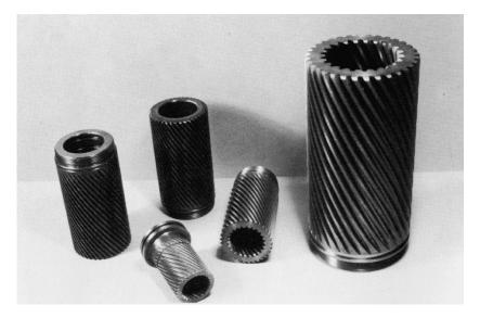
These are rotary actuator piston sleeves made of V–4 (80–55–06) ductile iron. These worm gears are grooved on the O.D. and I.D. The O.D. is then threaded with ring grooves placed on both O.D. and I.D. This part shoes how VERSA–BAR fits even in the most complex machining application.
