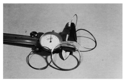
During our machine testing for this guide, sample rings were routinely parted as thin as .010 thick. This demonstrates the superior metallurgical integrity of the VERSA–BAR con–cast product.
